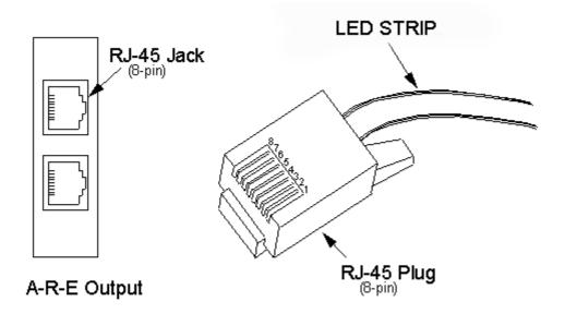
b. In case you have a quad LED strips unit, connect two LED strips to each RJ45 connector on the A-R-E interface, via the RJ45 splitter provided in the expansion package.
